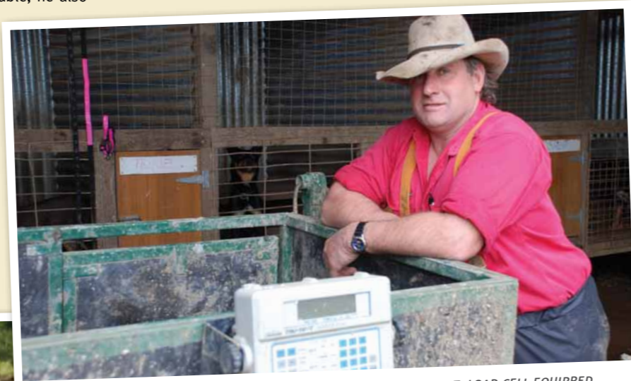
SCOT WEIGHS ALL HIS STUD CALVES AT BIRTH USING THIS LIGHT WEIGHT, LOAD CELL EQUIPPED TRAILER TOWED BEHIND THE QUAD BIKE. KENNELS FOR HIS KELPIE BREEDING OPERATION CAN BE SEEN IN THE BACKGROUND.
